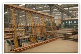
Large glass sheets can now easily be loaded onto the laminating line. Hydraulic cylinders bring the table into a vertical position for easy glass sheet loading.
