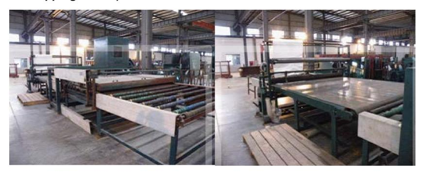
A washing machine is connected with the backing process ensuring a clean and dry mirror surface.
